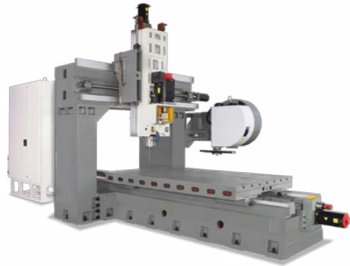
STYLE DC-BL type BL type is executed with block guiding on the X-, Y- & Z-axis.
